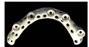
Laser melted implant sub frame for denture case.
