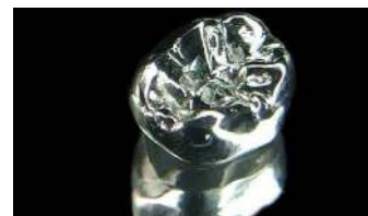
Full metal laser melted crown.
